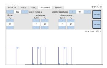
First of all, you should set the water target which you would like to produce. This value will not be exceeded. Varying the bloom or the turbulence phase will adapt the development phase automatically. The development phase itself is self-adjusting between duration and flow ratio of its pulses. Depending on how detailed you would like to compose your recipe, the display resolution can be set 1 or 0.1.
