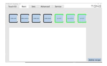
For the coffee recipes, the brewing temperature and the pulsation of the water flow is pre-defined, based on the experience of TONE coffee experts. You can simply adjust the amount of water (click or click and hold on the arrows) and choose between cone and flat filters. Make sure you have installed the correct spray head insert for each filter type. For the cones you need to install the insert with 5 holes, for the flat filter the insert with 18 holes.
