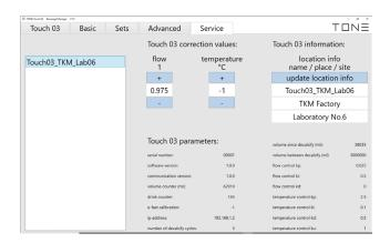
In case your brewer should extract more or less water than intended you can tweak the flow rate by setting a value below 1 in case you want to reduce the amount of water or a value above 1 if you want to increase the amount of water. This is a very sensitive tool an can only be adjusted in permille steps.
