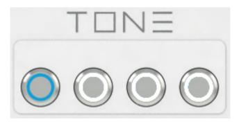
Blue chasing light (Button 1-4) after switching the brewer ON and after finishing a recipe
